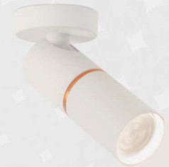
PLAFON / SPOT SCOPE MINI SHORT 1087 Porta lâmpada: 1 x GU10 MR11 Spot: Ø 38 x 145 mm Luminária completa: ↔ 145 x ↓ 55 mm Base de teto: Ø 60 x 15 mm
